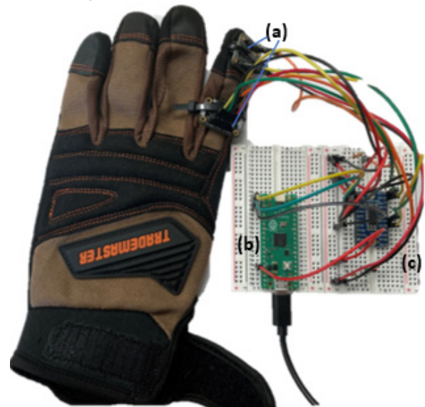
Fig. 1 Tremor measurement device with the (a) IMUs, (b) Raspberry Pi Pico microcontroller, and (c) multiplex
