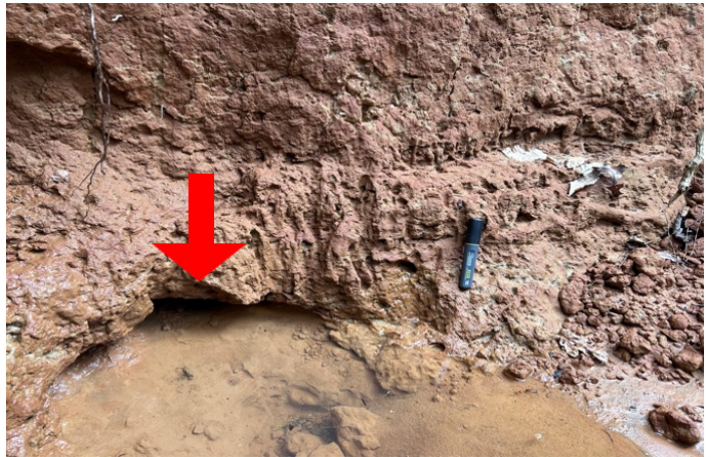
Fig. 1 Concentrated leak erosion at a site monitored in North Alabama by Dr. Jack Montgomery and students
