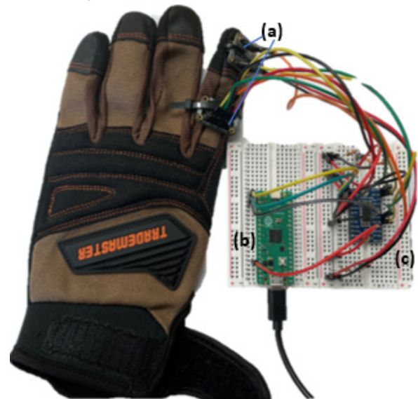
Fig. 1 Tremor measurement device with the (a) IMUs, (b) Raspberry Pi Pico and (c) multiplex.
