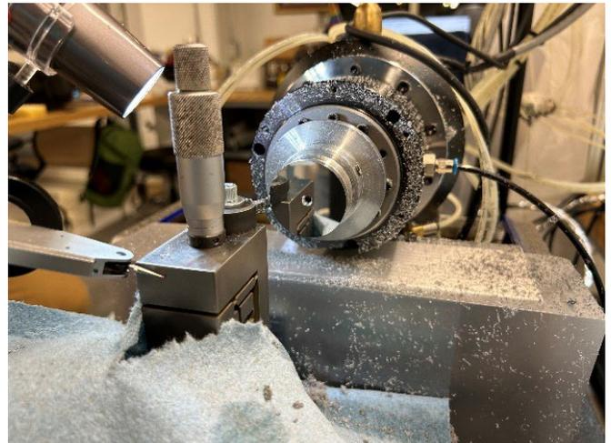
Fig. 1. Diamond turning a planar aluminum mirror.
