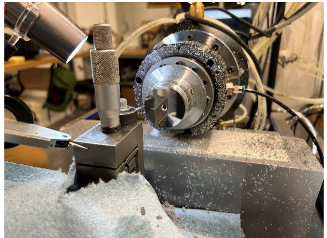
Fig. 1. Diamond turning a planar aluminum mirror.
