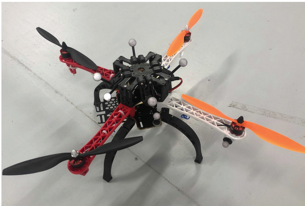
Figure 5. In-house assembled, soldered, and flight-tested quadrotor UAV with custom designed 3D printed parts and our own rc_pilot firmware.
