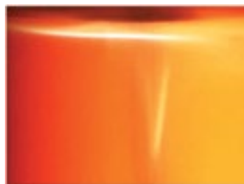
Figure 4b. Combustion of cetane pendant droplet at 800 °C.
