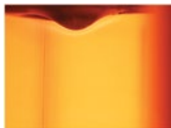
Figure 4a. Combustion of 70% aqueous glycerin pendant droplet at 900 °C.
