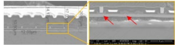
Figure 2. SEM images of the cross-sectioned e-mode GaN HEMT device showing the overall dimensions and transistor structure, with critical features indicated by arrows.
