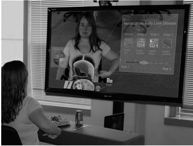
Figure 11.3 Mockup of a hypothetical AR mirror for diabetes nutrition education. Internal physiology and nutrition information are situated (i.e., visually registered) in real-time with the body and food. An embodied interaction (e.g., pointing) near the liver provides information at a different physical scale (e.g., cellular) and supports visual comparison of stages of the disease. Heads up display interface elements such as the slider allow exploration of body changes at different timescales . A plate of food provides input for the simulation . Selecting, portioning the food, and pointing with the fork are a tangible user interface . Such a hypothetical interface demonstrates the flexibility of AR HCI but leaves many unknowns for matching the design to suit a user’s needs.
