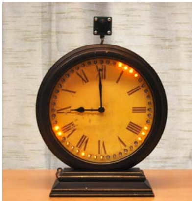
Figure 7.1 Activity clock. A technology that detects the older adult's motion and measures their level of activity.
