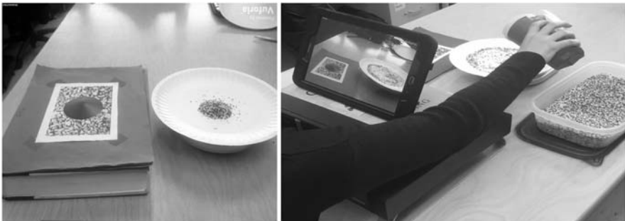
Figure 11.2 Augmented reality being used to show proper food portion sizes. The patterned paper on the left informs the AR system of what size cone to show when viewed through the camera on a tablet computer. The human tries to measure out a portion of quinoa similar to the goal amount shown by the cone (Matalenas, 2017). Thus, the contextual environment remains the same, save the addition of “augmented” information available via the computer. View of such AR can be done via tablets, smartphones, glasses, or any computer-mediated display.
