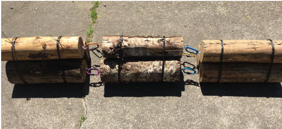
Figure 14 - Cable attenuator with carabiner connections.
