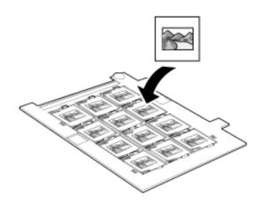
Place the film holder on the document table so that it is aligned with the upper right corner.
