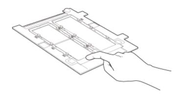
Place the film holder on the document table so that it is aligned with the upper right corner.
