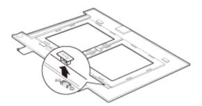
To return the film holder to its default height, 0.12 inch (3 mm), place the film height adjusters so that the arrow on the adjusters face the O symbol on the bottom of the film holder.
