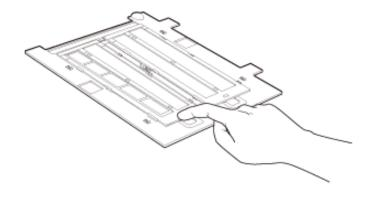
Place the film holder on the document table so that it is aligned with the upper right corner.
