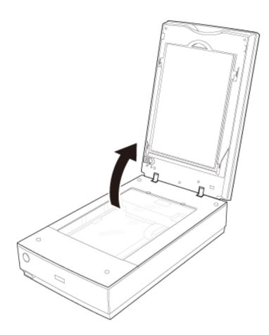
Pull the scanner cover straight up and off the scanner.
