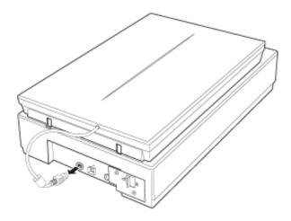
On the back of the scanner, slide the transportation lock to the locked position to secure the scanner carriage.
