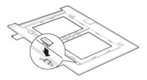
Remove all of the film height adjusters on the back of the film holder to decrease the height between the film holder and the document table to 0.1 inch (2.5 mm).
