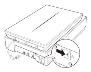
6 Attach the protective materials that came with the scanner, then repack the scanner in its original box or a similar box that fits the scanner snugly.
