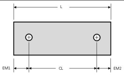
2. There are four more drawings on the next page. Nominally, all four should produce the same part. In reality, the tolerances will play a role in feature location. Fill in Table 2 with the maximum and minimum feature values that correspond to the pictures on the next page.
