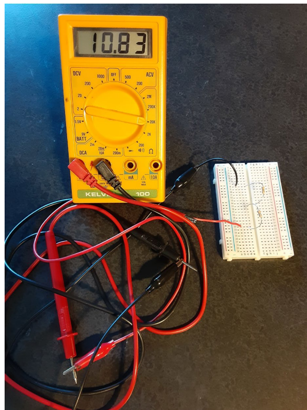
Figure 5: Measuring Series Resistors
