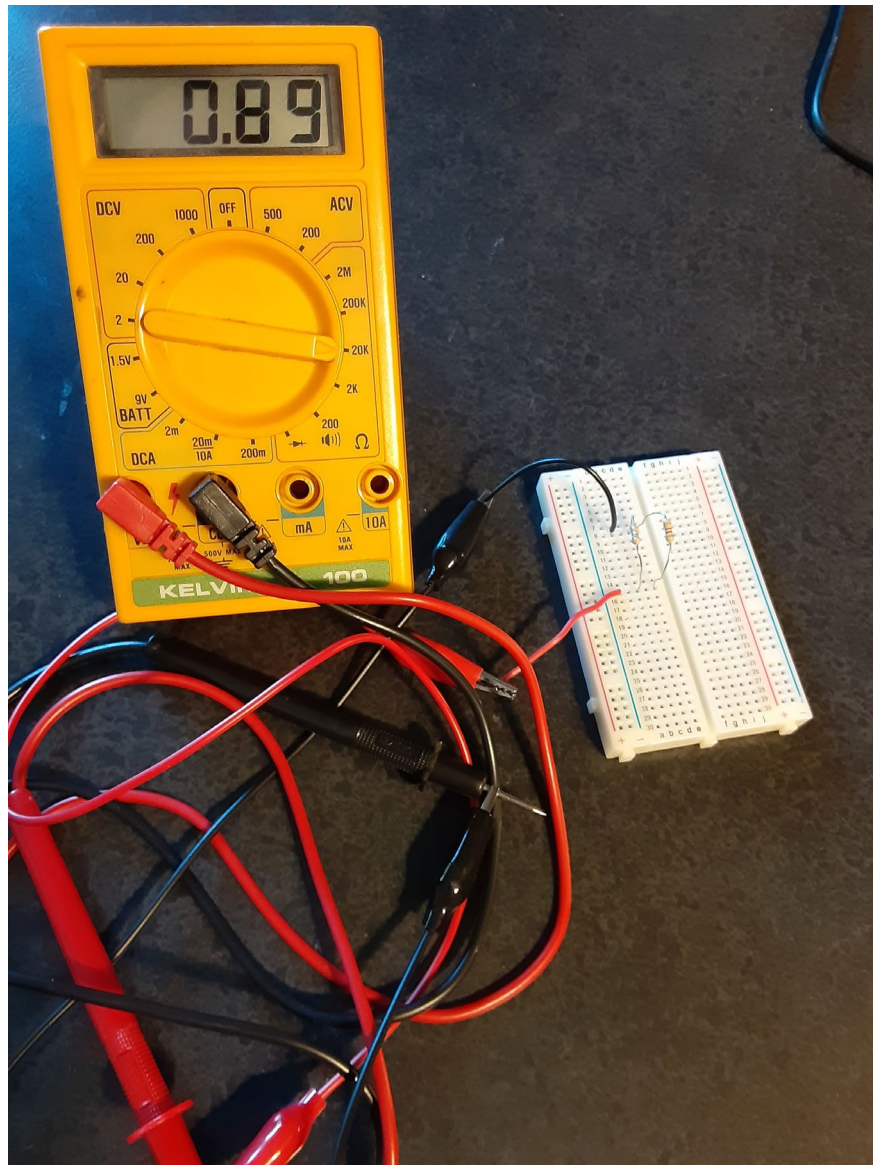
Figure 6: Measuring Parallel Resistors
