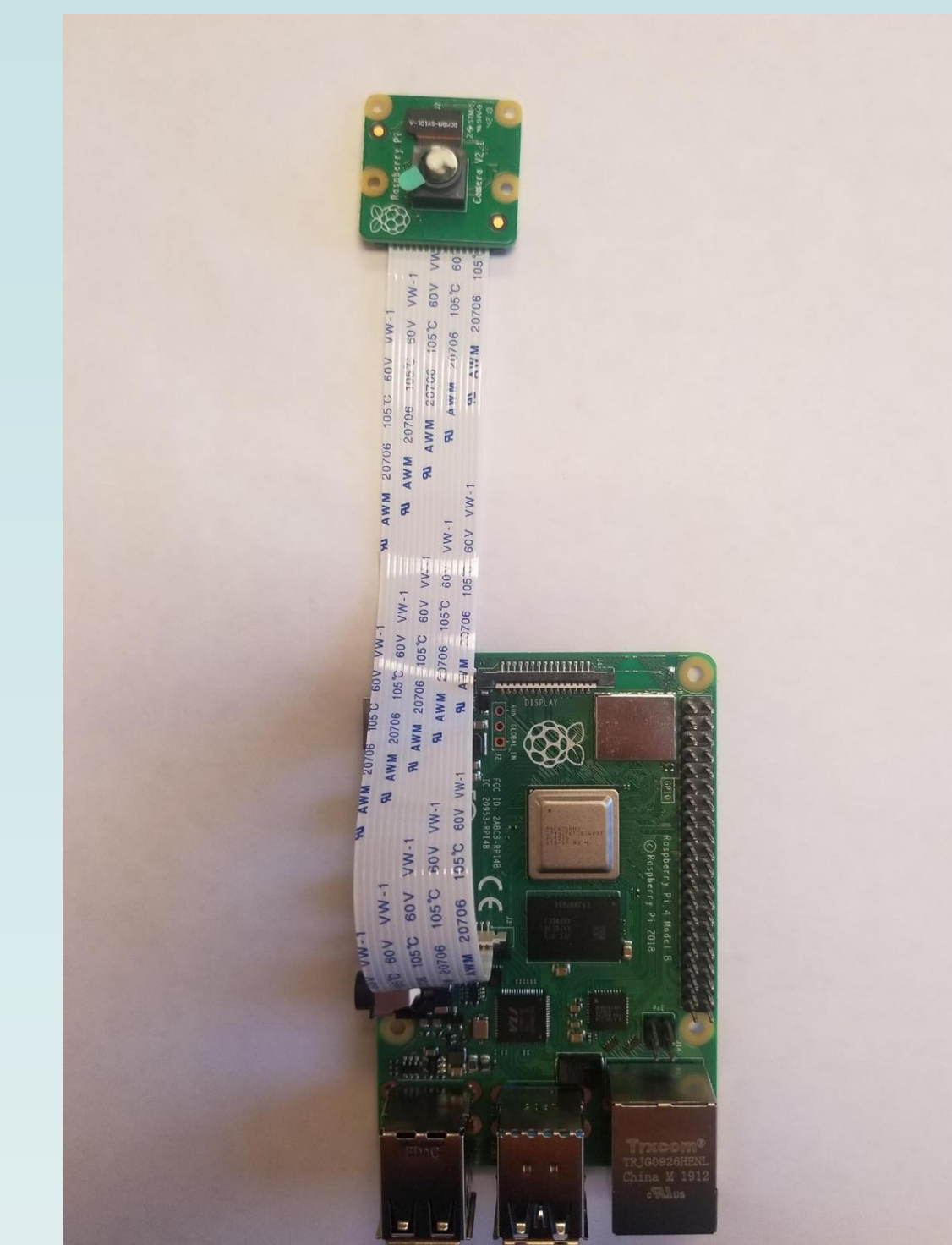
Figure 4. IoT Security Camera made using the Raspberry Pi 3.
