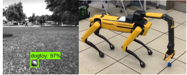
Figure 4. Successful Ball Detection and Pickup
