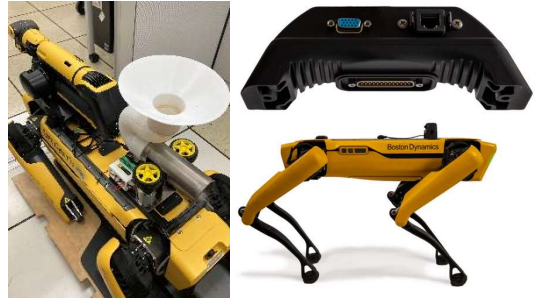
Figure 1. (Left) Spot Payload Prototype (Right) General Expansion Payload/Power Supply
