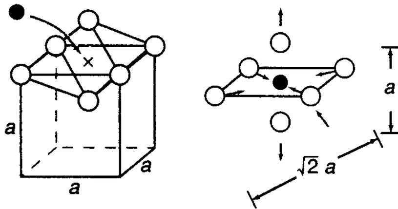
**Fig. 6.3** An interstitial atom in the octahedral site of a BCC lattice produces a tetragonal distortion.
