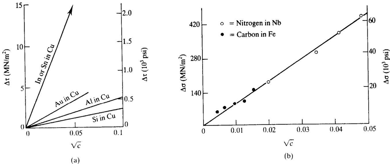
Verification of the  $c^{1/2}$  dependence of solid solution hardening
