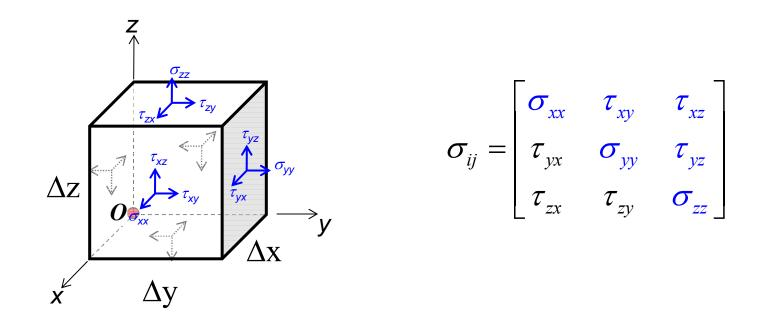
In three dimensions the state of stress is described by the stress tensor.
