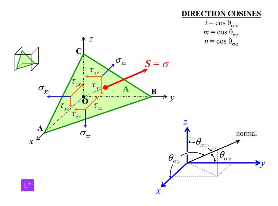
The components of s parallel to the original x-, y-, and zaxes (i.e., s<sub>x</sub>, s<sub>y</sub>, s<sub>z</sub>) are:
