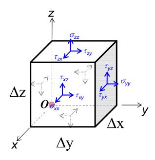
$$oldsymbol{\sigma}_{ij} = egin{bmatrix} oldsymbol{\sigma}_{xx} & oldsymbol{ au}_{xy} & oldsymbol{ au}_{xz} \ oldsymbol{ au}_{yx} & oldsymbol{\sigma}_{yy} & oldsymbol{ au}_{yz} \ oldsymbol{ au}_{zx} & oldsymbol{ au}_{zy} & oldsymbol{\sigma}_{zz} \end{bmatrix}$$
