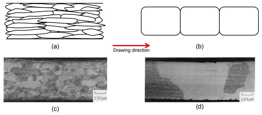
Schematic microstructures of (a) drawn W wire and (b) such a wire following high-temperature exposure. Figures (c) and (d) are light optical micrographs of W before and after high-temperature exposure.
