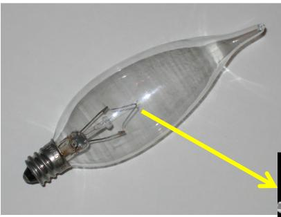
Tungsten light bulb filaments fail after a few thousand hours.
