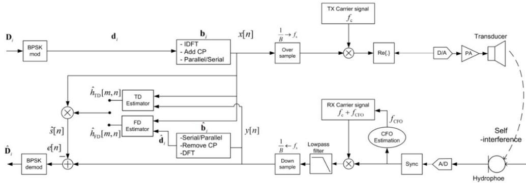
Fig. 6. UWA-IBFD transmission and reception procedure using OFDM signals.
