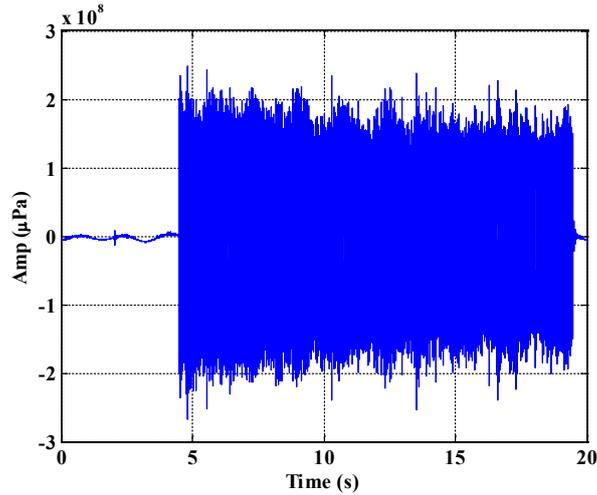
Fig. 4. The received passband BPSK signal from raw data “RBW1472\_20190709\_161000.wav”.
