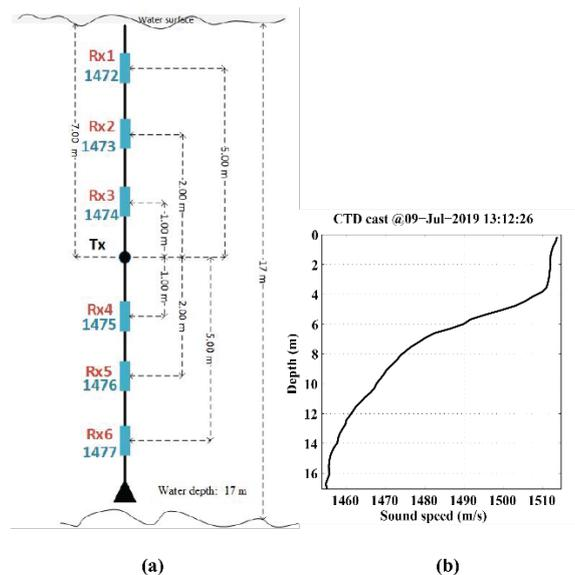
Fig. 3. (a) Experimental configuration at Lake Tuscaloosa. The water depth was 17 m. The transducer was installed at 7 m below the water surface. Six digital hydrophones were distributed along the mooring line. (b) Sound speed profile.
