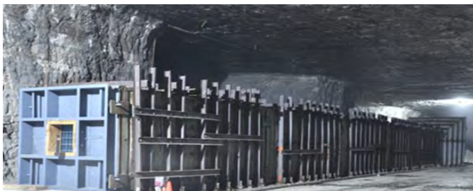
Figure 1: Underground mine with shock tube facility
