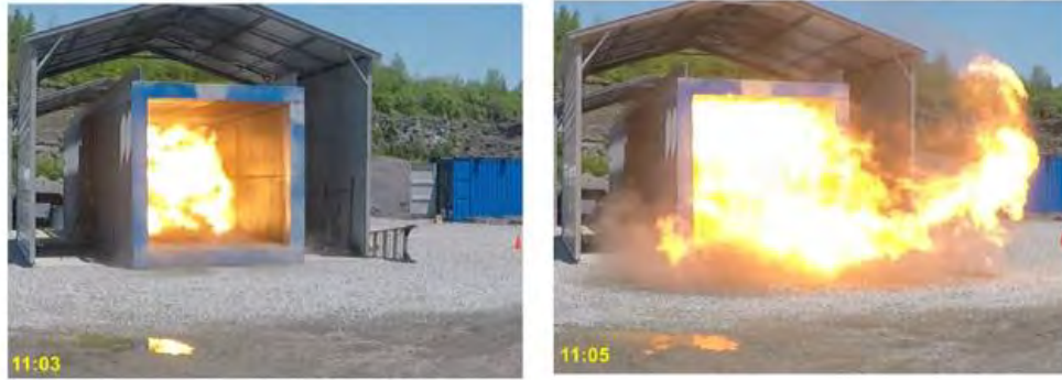
Figure 3: Methane and coal dust explosion test at UKERT
