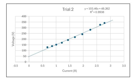
[Figure 2 is the graph of Voltage versus Current for the second trial, with the accompanying slope value.]
