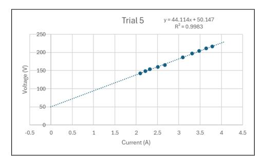
[**Figure 5** is the graph of Voltage versus Current for the fifth trial, with the accompanying slope value.]
