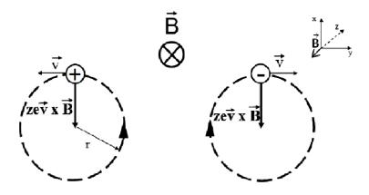
If the quantities for velocity, orbital radius, and external magnetic field can be measured, then the fundamental constant  $\frac{e}{m}$  can be calculated.
