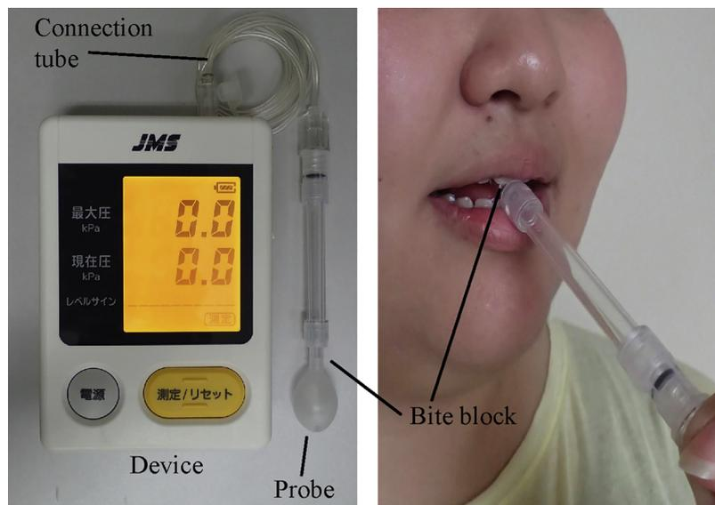
Fig. 1. JMS Tongue Pressure Measurement Device.
