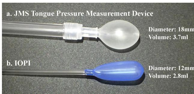
Fig. 2. Probes for tongue pressure measurement. a. JMS Tongue Pressure Measurement Device. b. Iowa Oral Performance Instrument.
