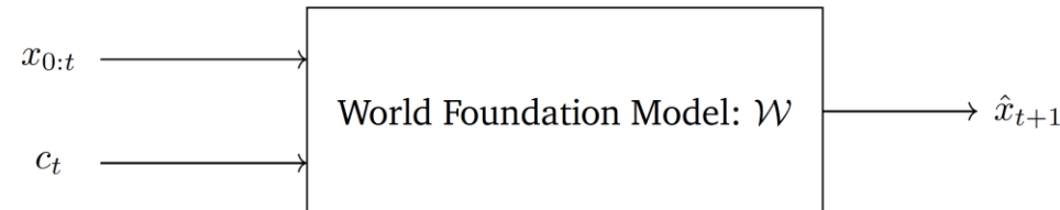
Figure 3: A world foundation model (WFM) \mathcal{W} is a model that generates the future state of the world x_{t+1} based on the past observations x_{0:t} and current perturbation c_t .
