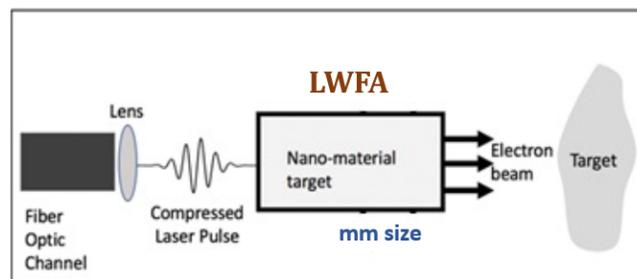
Figure 1.. Electron accelerator at the tip of an endoscope or colonoscope for targeted therapy after reference [5].
