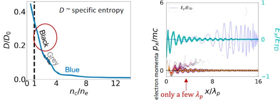
Figure 3. (Left) Regimes of plasma wakefields with various plasma density  $n_e$  with respect to critical density  $n_{crit}$ ; (Right) Plots with electron momentum, space-charge field along the laser propagation direction. From reference [8].
