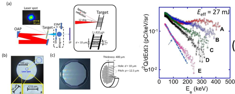
Figure 4. Near-critical density LWFA is experimentally verified. Charts are adopted from reference [8].
