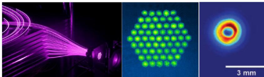
Figure 10. XCAN 61 channel CBC laser. The bundle of 61 YB doped 30 μm MFD amplifying fiber can be seen fluorescing. The fibers are arranged in the laser head in a honey-comb distribution and subsequently collectively collimated through a lenslet array (far right of the left image). Collective phase delays recording through interference pattern (right). Adapted from [ref. 19].
