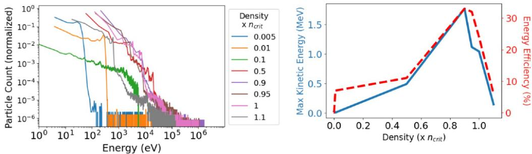
Figure 2. Electron energy spectra (left) and laser-electron conversion efficiency (right) with increasing plasma density towards the critical density, adopted from reference [7].
