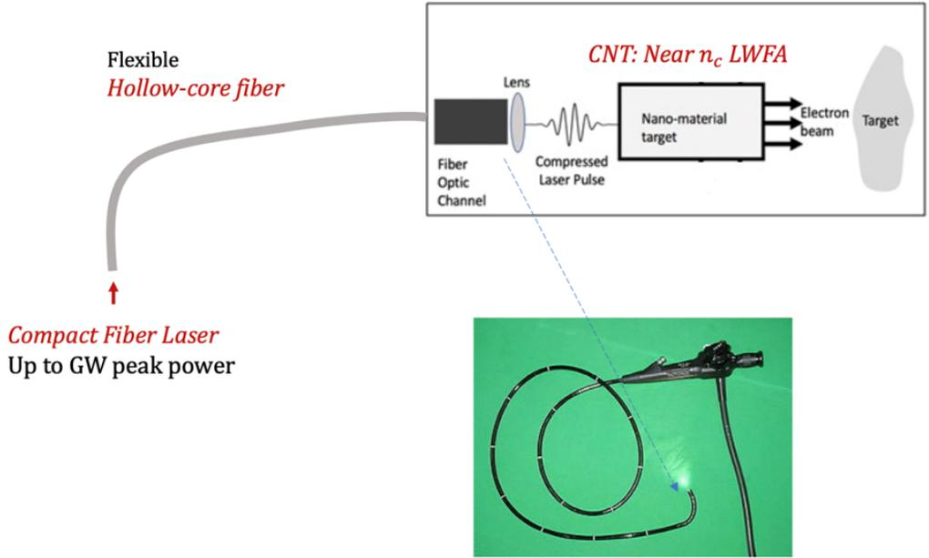
Figure 12. Implementation concept of the proposed endoscopic laser accelerator. A generic endoscope picture is used to aid the visualization of the concept apparatus.
