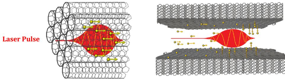
Figure 5. CNT's tube diameter can be flexibly produced to dial in critical density after reference [8] Laser pulse size not proportional to CNT.
