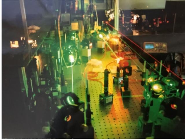
Figure 7. Femtosecond dye laser system which produced 100 fs, 200 mega-watt peak power. Focused beam had  $10^{14} \text{ W/cm}^2$  peak intensity [14,154]
