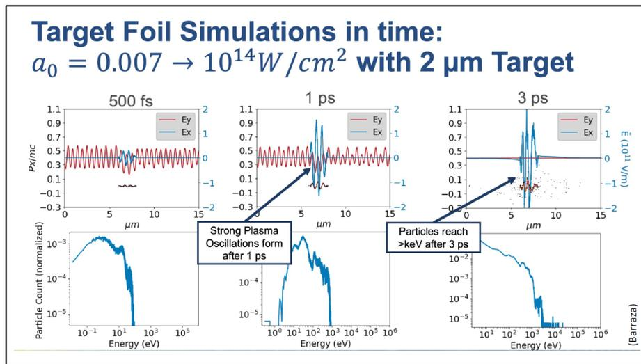
Figure 6. Laser parameter, wakefield magnitude, electron momentum and energy from beat-wave LWFA simulations for endoscopic accelerator. Studies are given in reference [7]. This plot is from private communication with E. Barraza.
