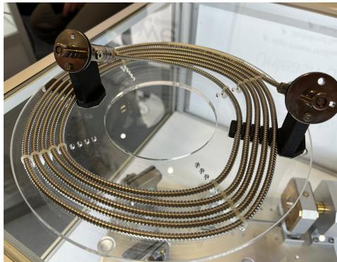
*Figure 11. A hollow-core fiber example by PT Photonics Tools [ref.26b]. One end is the launch and the other end is the delivery point where microscopic accelerator can be placed, perspectively, inside a patient's body. Bending radius is about 25 cm, quite realistic for the application. (Photo with PT Photonics Tools permission)*
