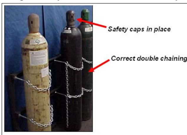
Figure 6.3 – Cylinders Stored and Chained Correctly
