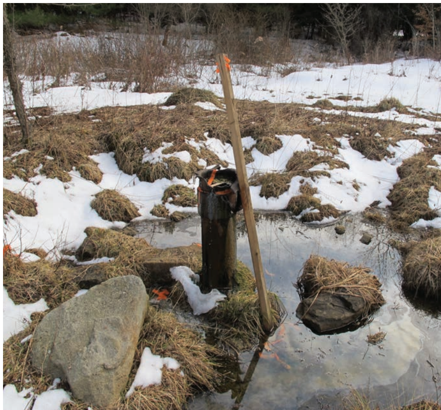
Image 18: Abandoned gas wells leak methane and other GHGs to the atmosphere and a program to identify and plug them with resulting offsets is being developed. Credit: Susan Phillips / StateImpact Pennsylvania
